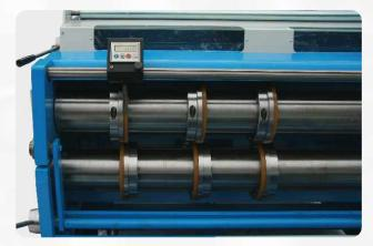
Plate twisting is prevented by urethane rings in slitting rolls. Digital measuring device makes aligning easy, accuracy 0,1 mm
